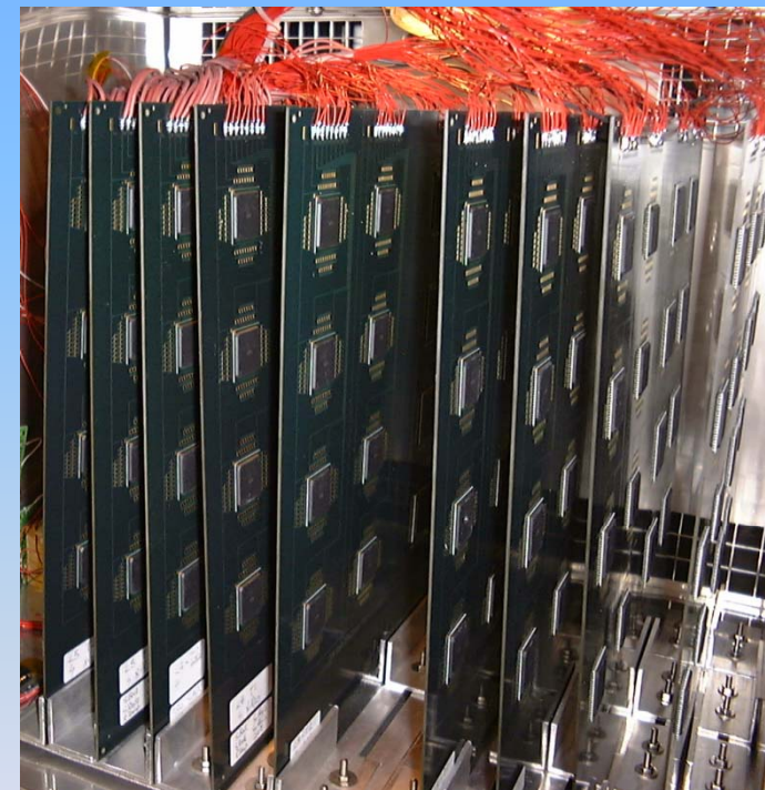
Test Boards in Thermal Cycling Chamber
