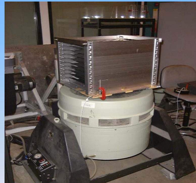
Specimens on the Shaker (Vertical Vibration)
