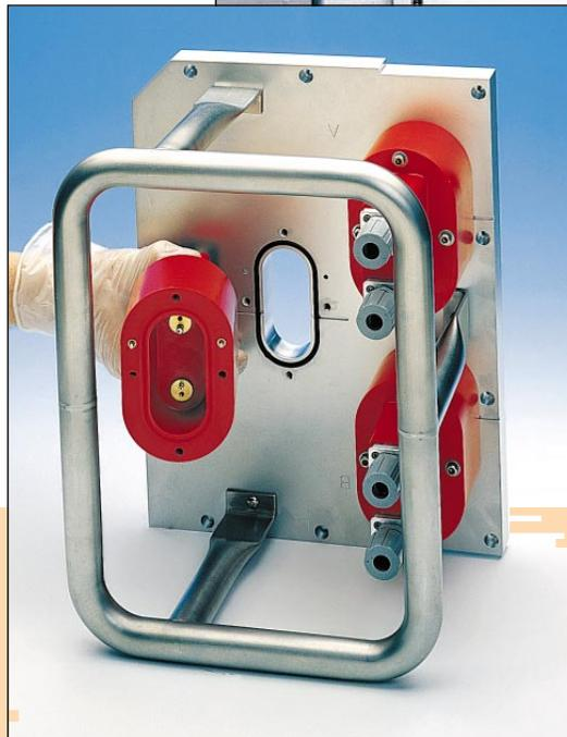
Mistakeproofing ideas such as this handle make it easy for workers to pick up the assembly for a particle accelerator from Varian Ion Implants Inc., Gloucester, Mass., and set it safely on its side or end without damaging electrodes. Workers must insert the assembly into the vacuum chamber without damaging delicate graphite parts. To do so unerringly, the vertical tab on the foreground plate and notch in the mounting plate make it impossible to incorrectly insert the assembly.
